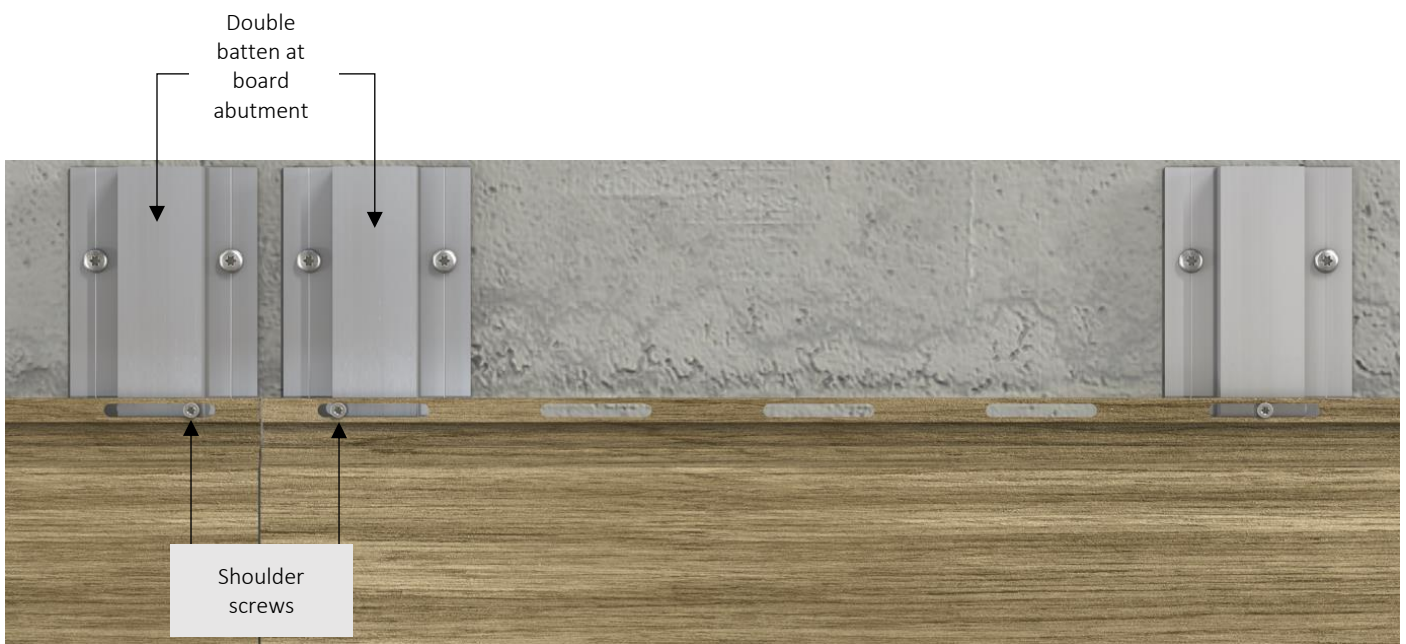
FRONT ELEVATION LYNX HORIZONTAL SIDING
