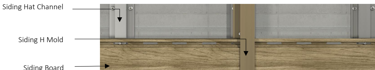
Gap Siding Spacing Ref. Table 1.4
