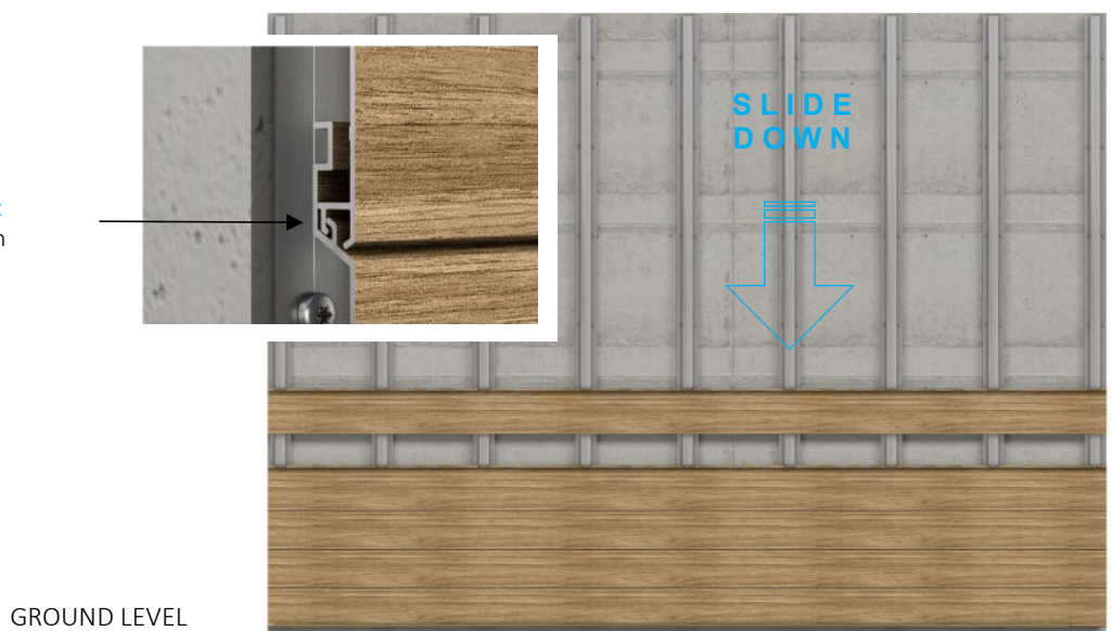
FRONT ELEVATION LYNX HORIZONTAL SIDING
